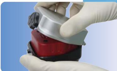
Sterile scrub technician closes battery housing lid and secures locking knob.
