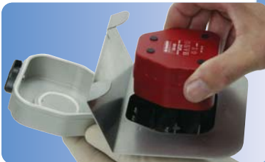
Circulating nurse presses the non sterile battery into the battery housing.
