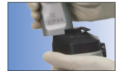
Sterile nurse locks aseptic battery housing into the handpiece.
